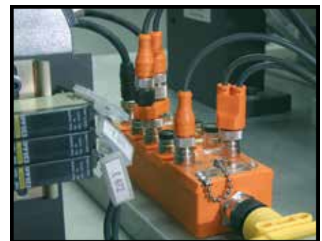
Module depicted with M12" bus connection and on-board 7/8" power auxiliary power connection with T-Connector.
